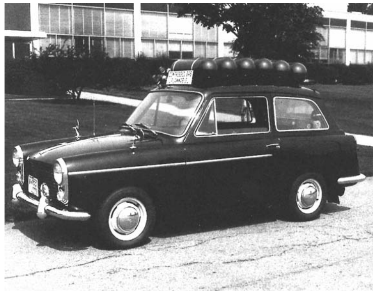
the converted Austin A40 with tanks on the roof, 1970
