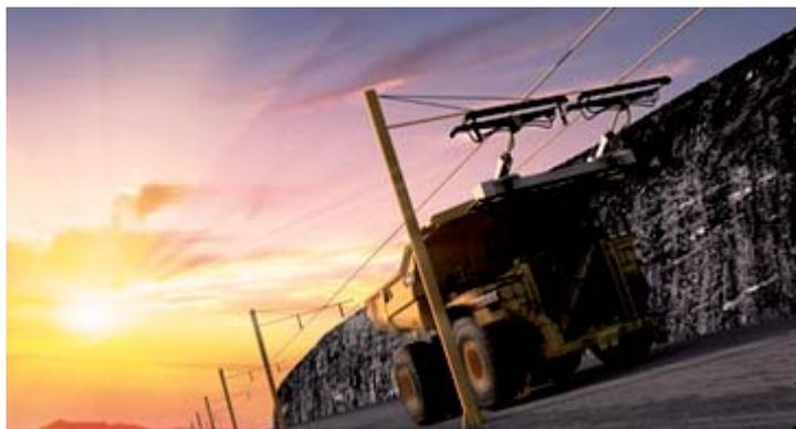
Figure 3: Illustrated, an electrified mine truck in the Aitik mine
