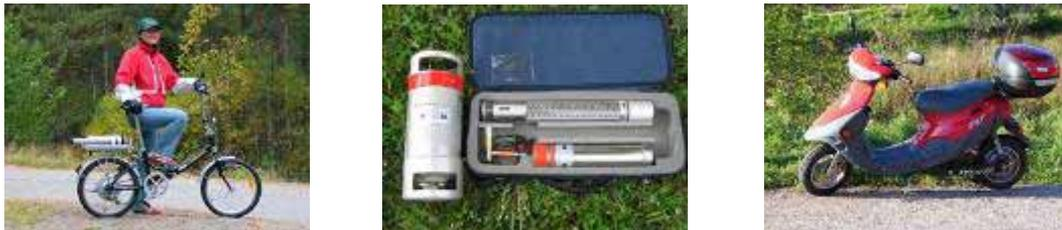
Fig. 11.3 Fuel cell HC-100 by Hydrocell Ltd combines metal hydride hydrogen storage and fuel cell to produce 14,4 V (DC) at 1,6 A current level. Hydrogen capacity of the smaller hydride storage MH200 is 36 Ah, and the larger unit MH1200 equals 220 Ah. These are used to power an e-bike and an e-scooter (photos by Hydrocell Ltd).
