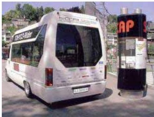
Fig. 16.2 TOHYCO Rider shuttle bus at inductive charging station (photo supplied by Muntwyler Energietechnik AG).
