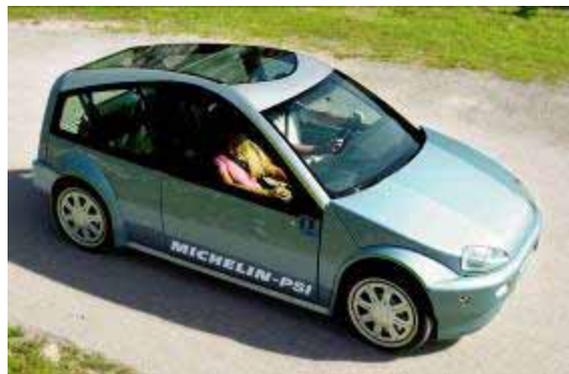
Fig. 16.1 HYlight fuel cell prototype vehicle by the Paul Scherrer Institute together with Michelin (photo supplied by Muntwyler Energietechnik AG).
