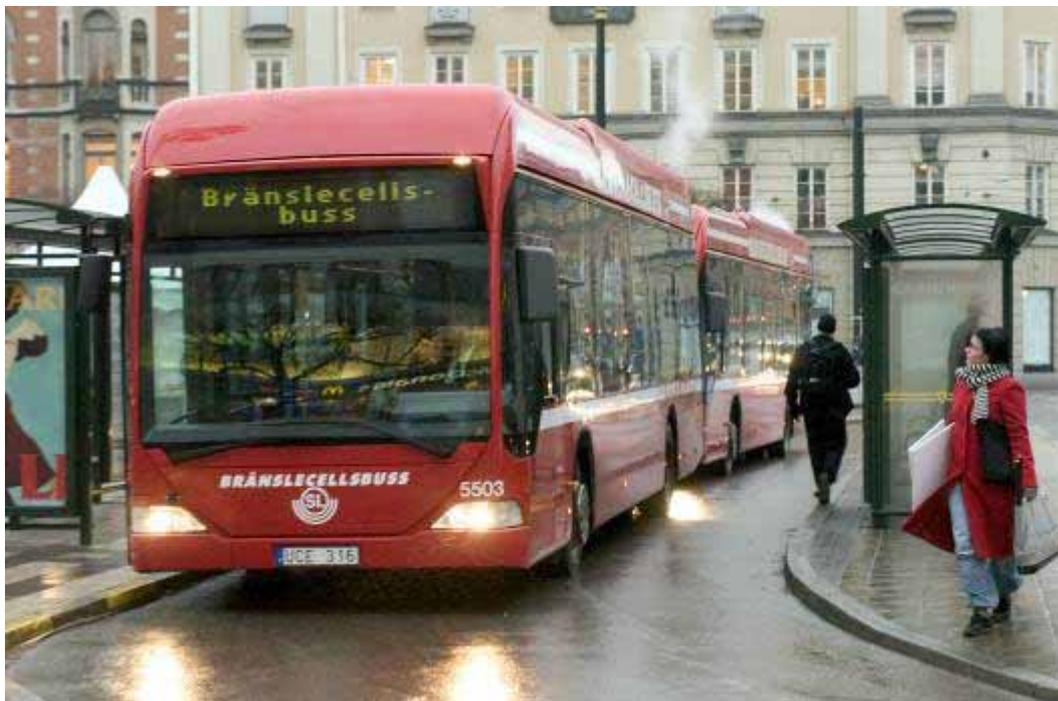
Fig. 15.1 The fuel cell version of an Evobus Citaro bus in service in Stockholm. (Photo supplied by STEM.)
